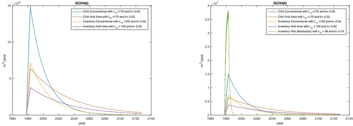
(a)  $Q_{CH_4}(t)$  in  $\frac{m^3}{yr}$  When Bioreactors Are Not Present Using Default Parameters in (3.1.1) and (3.1.2)
