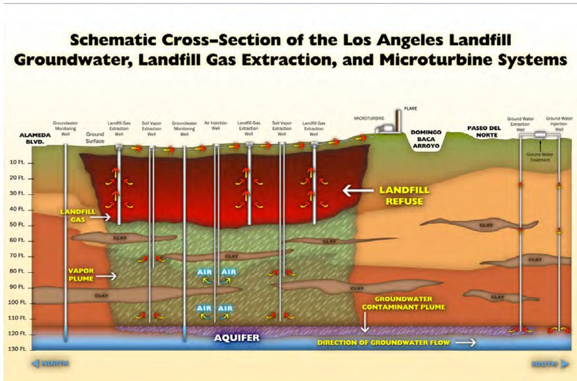
Figure 1.1: Schematic Cross-Section of the Los Angeles Landfill Groundwater, Landfill Gas Extraction, and Microturbine Systems
